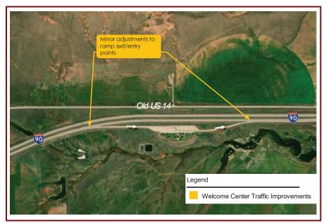
At MRM 1, the addition of a reconstructed rest area/welcome center would necessitate minor adjustments to the ramp exit/entry points. No other improvements would be anticipated.
