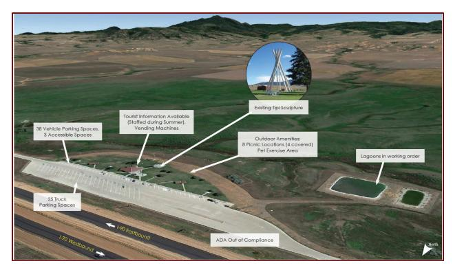
Figure 13 – Site details at the Existing Rest Area Location (MM 1)
