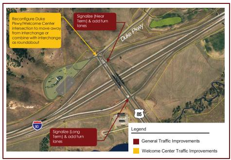
At Exit 17, construction of a rest area/welcome center would necessitate a reconfiguration of Dule Pkwy/Welcome Center intersection. The remaining improvement suggestions are due to general traffic growth in the area.
