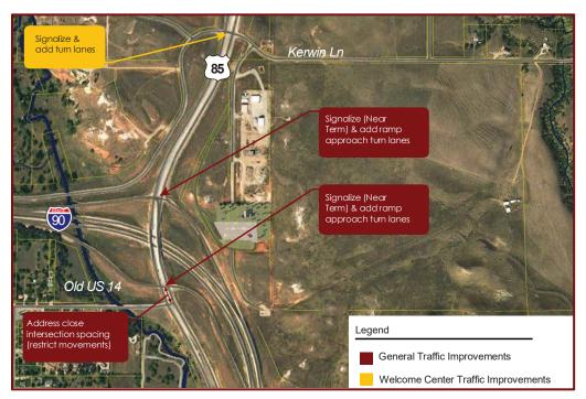
At Exit 10, construction of a rest area/welcome center would necessitate signalization at US 85/Kerwin Ln. The remaining improvement suggestions are due to general traffic growth in the area.
